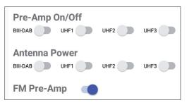
Recommendation: Turn on the pre-amplifier only when the input signal level is too low (below  $60 \text{ dB}\mu V$ ). Users may consult the automatic power level measurement of the input signal when adding a channel on the ONE Compact.
